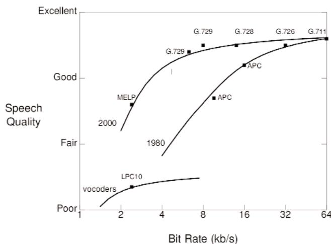
The figure shows the variation in speech quality as a function of bit rate. The coders labeled G.711, G.726, G.728, and G.729 were standardized by International Telecommunication Union (ITU). MELP and LPC10 are standardized coders for secure voice communication.
