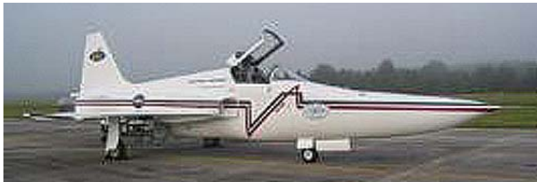
Shaped sonic boom demonstrator
